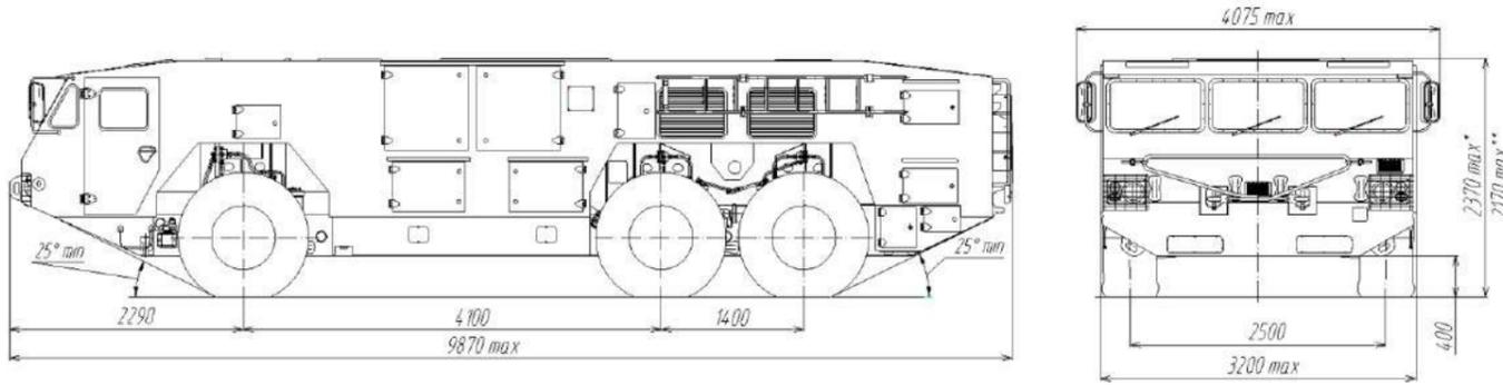
Family of highly-unified box-type chassis MZKT-6922 is intended for mounting and transporting of special equipment on all kinds of roads and terrains. Common base chassis allows to considerably simplify operation, maintenance, repair, reduces range of spare parts and number of maintenance staff
